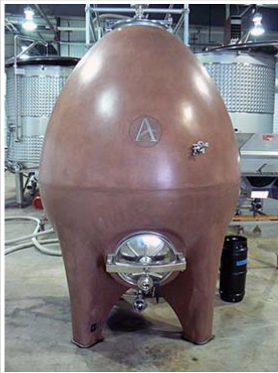
A concrete fermentation egg is part of the winemaking array.
