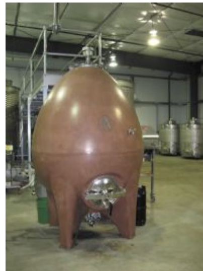
The egg-shaped fermenter holds 500 gallons of fermenting must at Andis Wines in the Shenandoah Valley. Photo courtesy of Deborah Budrick.
